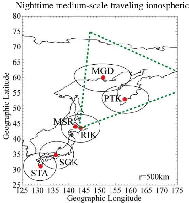
Figure 1. Stations of the all-sky airglow imagers, magnetometers, and the Hokkaido HF radar in Japan and Far-Eastern Russia. The circles and the triangle show the field of view of the airglow imager and the radar, respectively.
