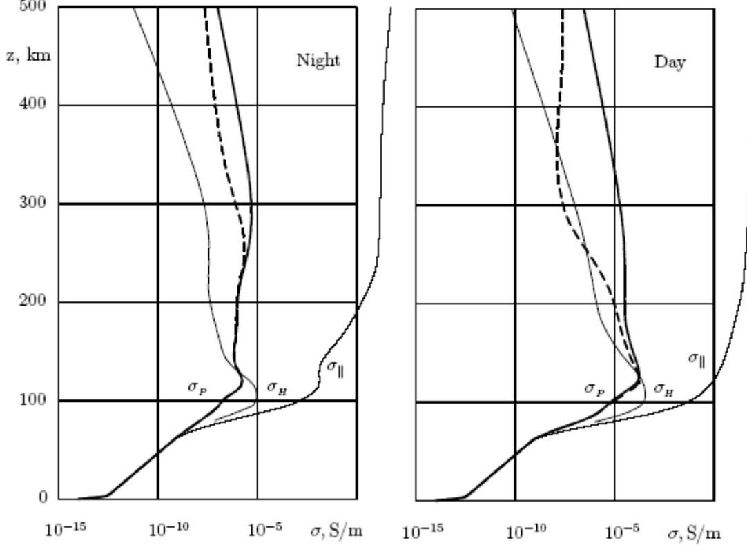
Fig. 1. Typical height distributions of the conductivity tensor  $\hat{\sigma}$  components in middle latitudes.
