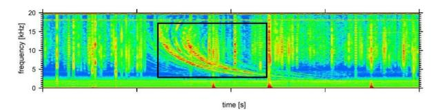
Fig. 1. Whistler typical imaging in spectral-time diagram of VLF signal.
